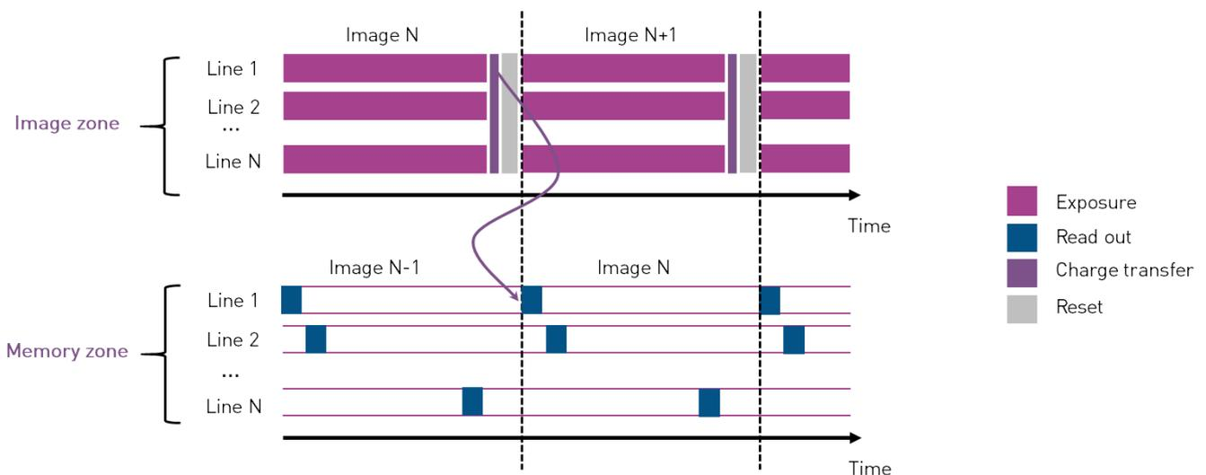
The acquisition mode is an intrinsic characteristic of the camera. However, it is important to understand the differences that will occur in an experimental context when using a camera with rolling or global shutter.
