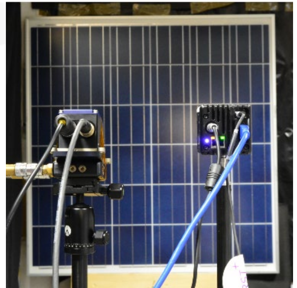
Laboratory set-up using a C-RED 3 camera (right) and a laser module (left) for photoluminescence imaging of a PV panel
