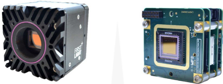
C-RED 3 camera in housed (left) and OEM (right) formats
