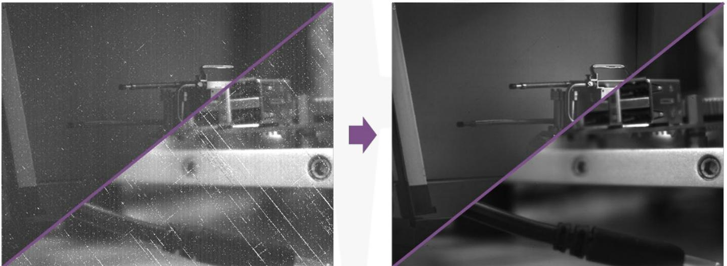
*Images before and after applying the full correction process on a C-RED 2 ER 1.9 $\mu\text{m}$  (top) and a C-RED 2 ER 2.2  $\mu\text{m}$  (bottom).
