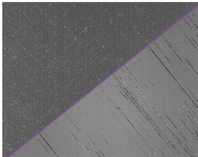
*Raw image acquired in dark conditions with a C-RED 2 ER 1.9µm (top) and a C-RED 2 ER 2.2µm (bottom). Acquisition parameters: medium gain, 600 fps, integration time 1.66 ms.*
