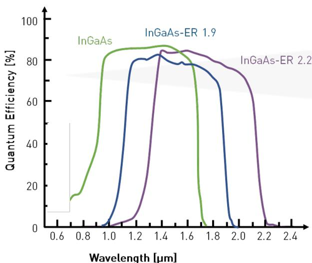
*Comparison of the quantum efficiency curves for cameras based on standard InGaAs and extended range InGaAs (typical values).*
