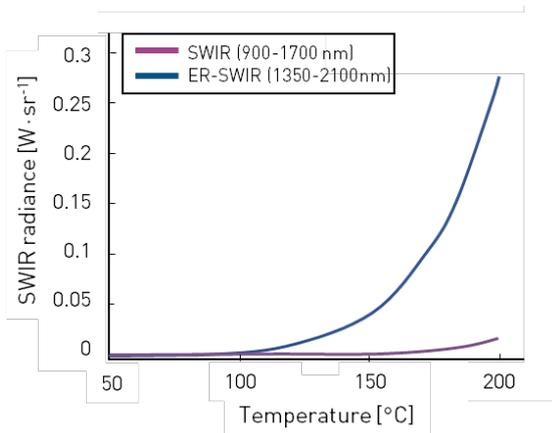
As a general rule, the error on a temperature measurement is higher for higher temperatures at longer wavelength. Hence, the SWIR and ER-SWIR ranges are better than MWIR or LWIR at temperatures within the range 300°C to 1600°C. ER-SWIR, contrary to SWIR enables measurements at temperatures below 300°C thanks to the higher radiance.
