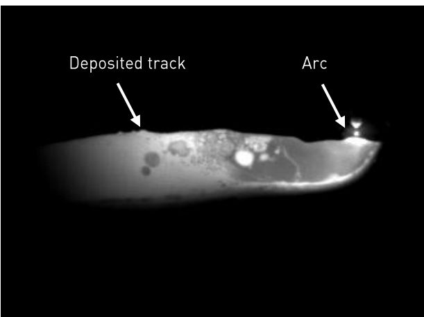
An electric arc is used as the power source to melt the metal wire. The homogeneity of the weld can be assessed in real-time.
