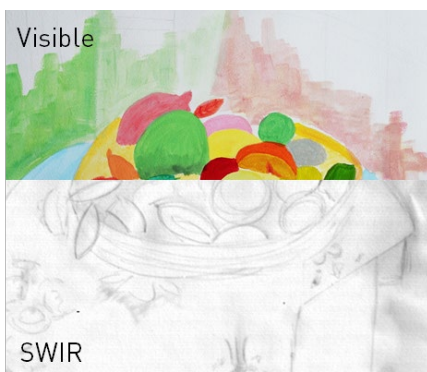
Visible and SWIR images of a water-based painting over a pencil drawing on paper. For SWIR imaging a non-stabilized C-RED 3 camera combined to a SWIR 16 mm lens is used. Integration time is 20 ms (50 fps) in low gain.
