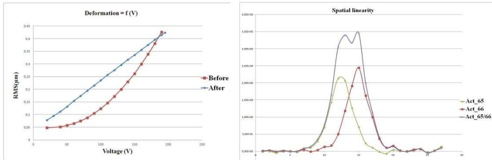
Figure 4. Left side: Graph showing mirror deformation as a function of applied voltage before (red) and after (blue) linearization process. Right side: Spatial linearity is shown (addressing both consecutive actuators is equivalent to their addition when addressing them individually).
