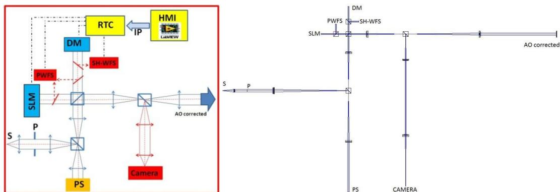
Figure 1. Left side: Schematic representation of LAM AO bench (left side). S (Source), P (Pupil), PS (Phase Screen), DM (Deformable Mirror), SH-WFS (Shack-Hartman Wave Front Sensor), SLM (Spatial Light Modulator), PWFS (Pyramid e Wave Front Sensor), RTC (Real Time Calculator), IP (Internet Protocol address) and HMI (Human Machine Interface). Right side: AO bench simulation under Zemax optics software showing the “low orders” and “high orders” correction floors and a third arm for imaging.
