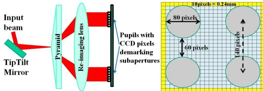
Figure 7. Left side : Pyramid concept. Right side: Example of desired design showing 4 sub-pupils (80 pixels each) located 10 pixels from the edge and separated by 60 pixels.
