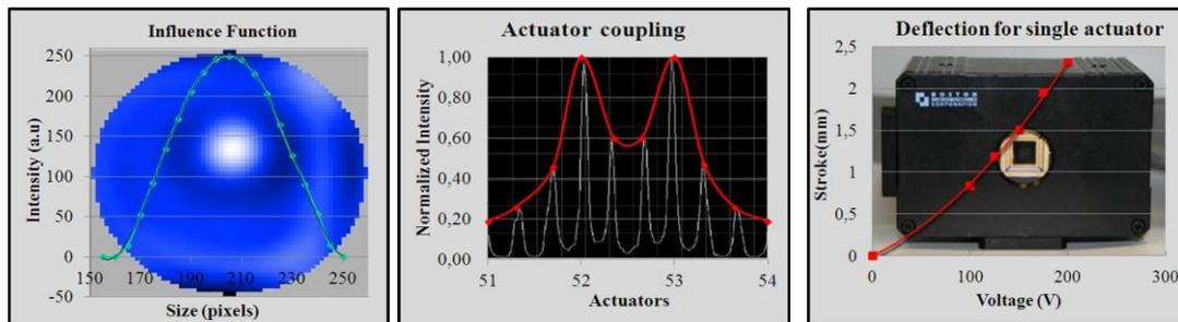
Figure 3. Left side: Influence Function shape. Center: graph illustrating an actuators coupling. Right side: Optical deflection.
