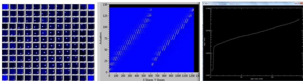
Figure 5. Left side : Influence functions for the 140 DM (12x12 without 4 corners) corresponding to a voltage of +/- 10 V. Center: Corresponding Interaction Matrix showing X and Y slopes (613x2). Right side: Graph showing the SVD (singular values decomposition) corresponding to the IM (conditioning factor is 15).
