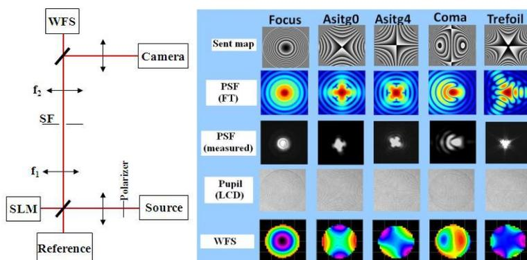
Figure 9. Left side : Schematic setup used for our SLM characterization. A reference mirror is used for comparison. Right side: Different SLM characterizations. Example of different maps (sent to the SLM) and corresponding measurements in the focal and pupil planes with the camera. The wave-fronts are also given in the pupil plane (WFS).
