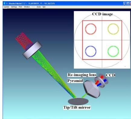
Figure 8. Pyramid concept design under Zemax. Inside figure represents the obtained sub-pupils on OCAM<sup>2</sup> detector (red square) .
