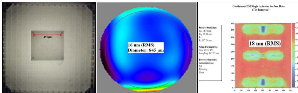
Figure 2. Left side : Boston 140-DM geometry. Center: surface data from MiniFiz interferometer. Right side: surface data obtained with ZYGO interferometer.
