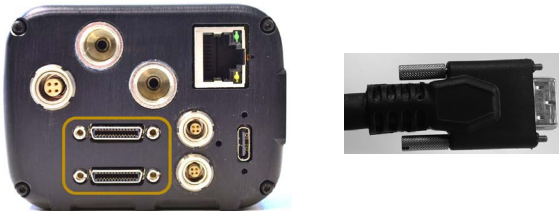
Fig. 6 : On the left, C-RED 2 back view. The yellow box shows the female Camera Link® connectors. On the right, a picture of one male SDR-26 Mini Camera Link® connector.
