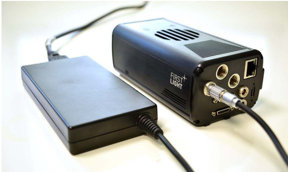
Fig. 8 : C-RED 2 with power supply connected thanks to the LEMO connector.
