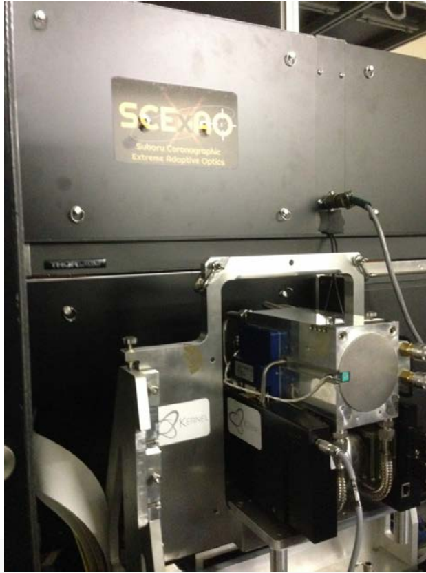
Fig. 4 : K-CAM: The KERNEL project C-RED-1 camera, is finally ready to observe on the IR side port of SCEAO. (Photo : F.Martinache, KERNEL)
