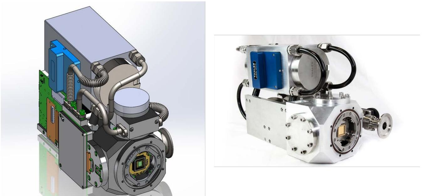
Fig. 7: the C-RED one infrared camera commercialized by First Light Imaging and that uses the Selex Saphira infrared array.
