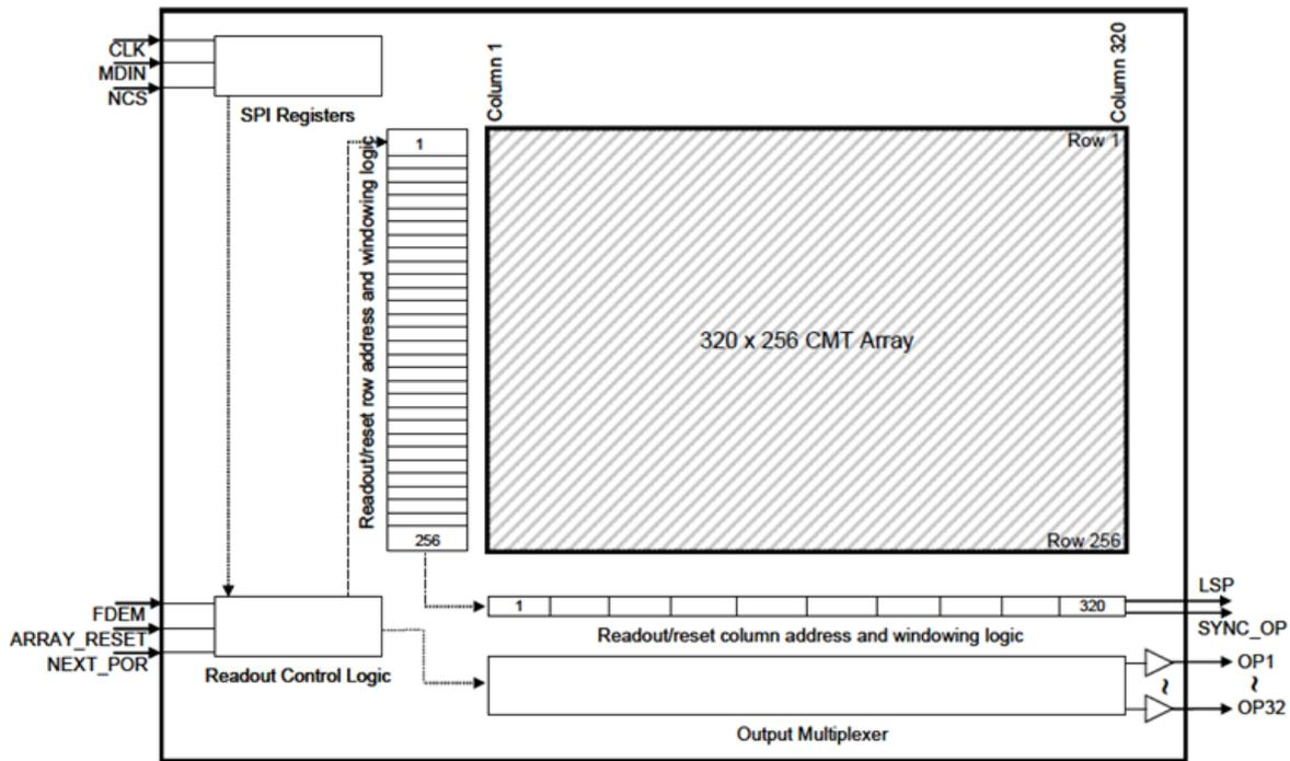
Fig. 8: the SELEX SAPHIRA ME1000 readout circuit architecture.
