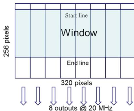
Fig. 1: The 1.6 kfps RAPID e-APD infrared detector configuration: 8 outputs 320 x 255 pixels with 30  $\mu\text{m}$  pitch. A rectangular window with programmable start line and end line can be defined to speed up the frame rate.
