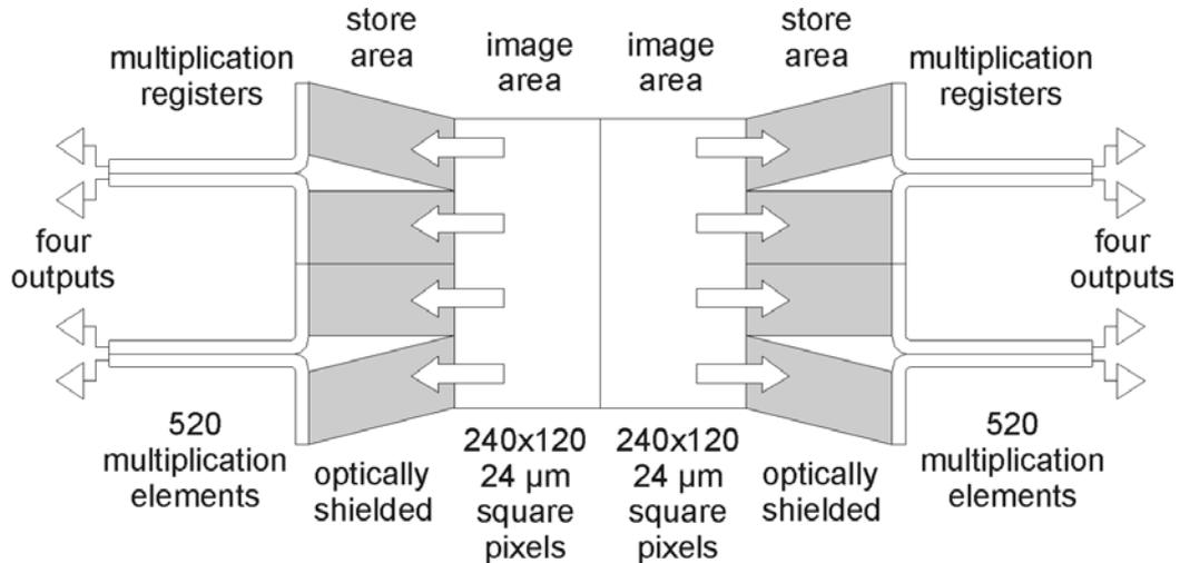
Fig. 13: Schematic of e2v technologies 240x240 pixel L3Vision CCD220. Eight Electron-Multiplying (gain) registers are used to obtain sub-electron noise at frame rates of 1300 fps.
