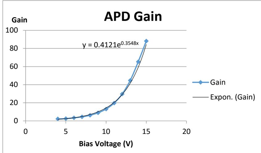
Fig. 10: Measured APD gain vs polarization voltage of MARK 13 array and exponential fit.
