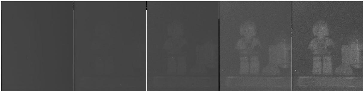
Fig. 12: Low light scene imaged with gains of 1,6,13,45 and 90 (from left to right) showing only a few defective pixels at high gain (<10 defective pixels) on our engineering grade device, CDS readout at 1700 FPS.
