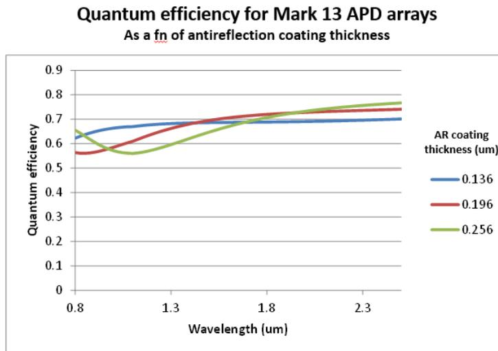
Fig. 9: AR coating and QE optimization for J, H or K bands of Mark13 e-APD diodes.
