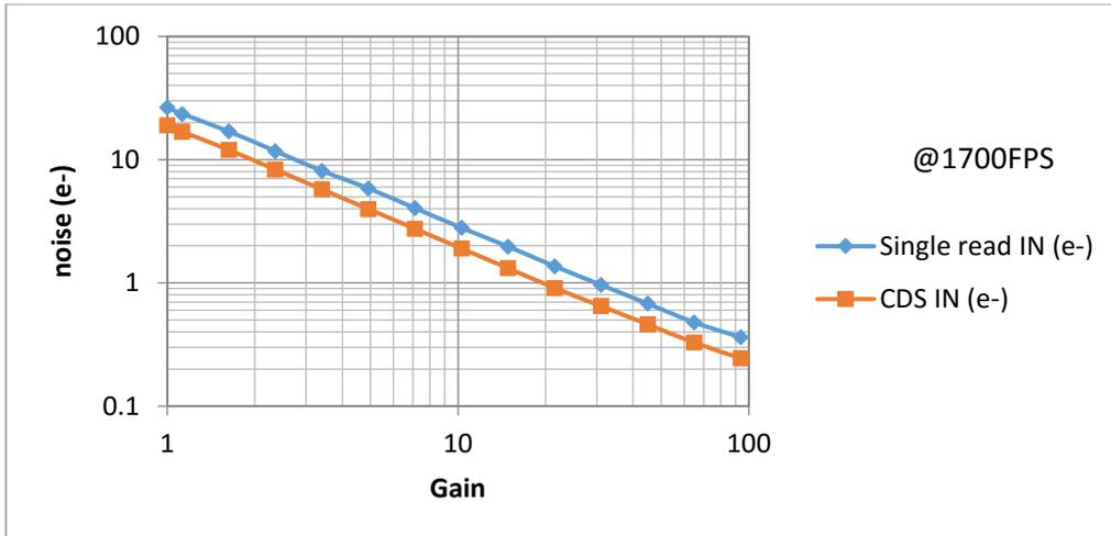
Fig. 11: Measured input referred readout noise vs APD gain for single readout and CDS readout.
