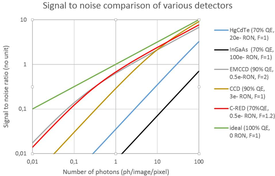
Fig. 14: Signal to Noise comparison of various detector technologies. CCD and EMCCD are sensitive in the visible. They are compared with IR detectors (InGaAs, slow scan HgCdTe and the C-RED e-APD camera).
