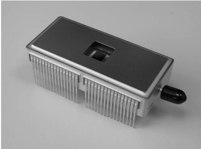
FIG. 4.—Photograph of CCD220 package with integral Peltier cooler that has been verified (first by thermal modeling, then by measurement) to cool the CCD below -45^{\circ}\text{C} to achieve <0.01 e^{-} \text{ pixel}^{-1} \text{ frame}^{-1} total dark current. See the electronic edition of the PASP for a color version of this figure.
