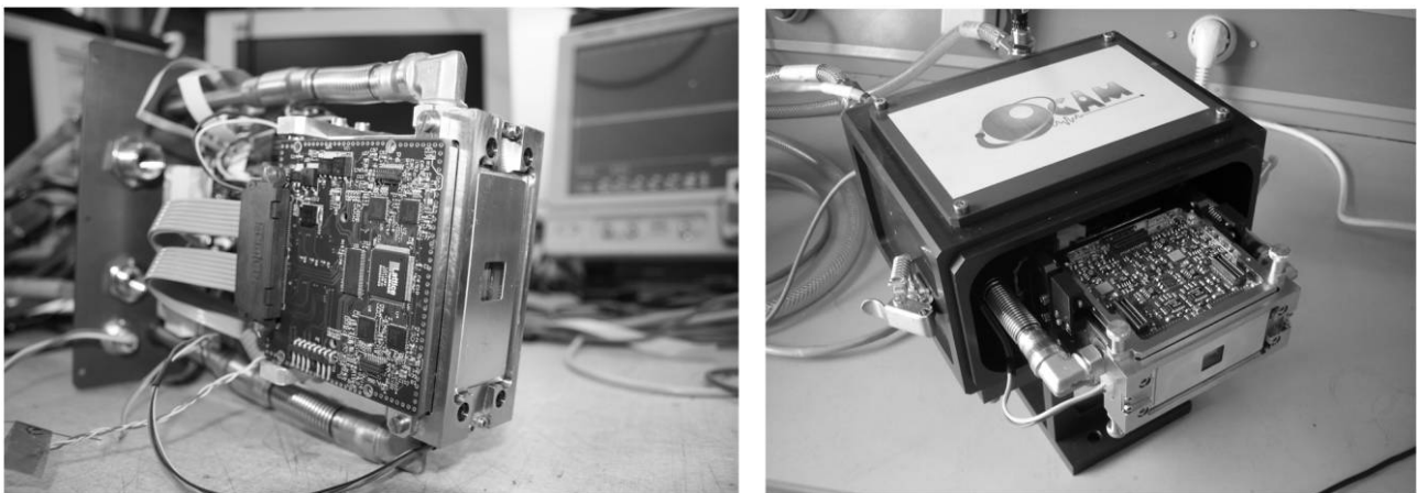
FIG. 6.—OCam controller views showing the front-end electronics as close as possible to the CCD220. See the electronic edition of the PASP for a color version of this figure.
